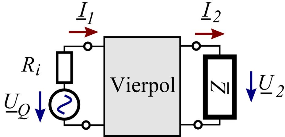
$$\begin{pmatrix} \underline{u}_0 - R_I \cdot \underline{i}_1 \\ \underline{i}_1 \end{pmatrix} = \underline{A} \cdot \begin{pmatrix} \underline{Z}_L \cdot \underline{i}_2 \\ \underline{i}_2 \end{pmatrix}$$
